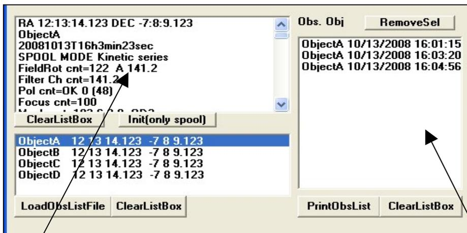
The init procedure is logged in the left listbox. Scroll through and check For errors (EMCD out of range etc, invalid sub image definition etc...) Also check that correct camera is selected (camera1 camera2 expert mode)
